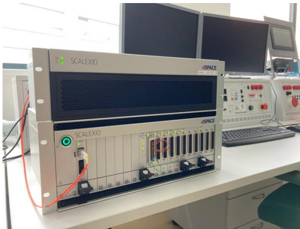
Workplace for the training - dSPACE Scalexio system with LabBox, dynamometer and tested motor
