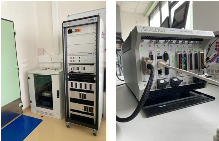
Hardware equipment which is going to be used for training 2 – dSPACE HIL and dSPACE AutoBox
