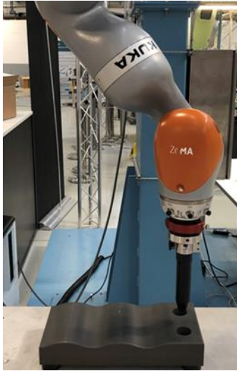
Sensitive robot performing a forced-controlled robot path
